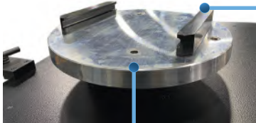
Pallet rails lock pallet to receiver
