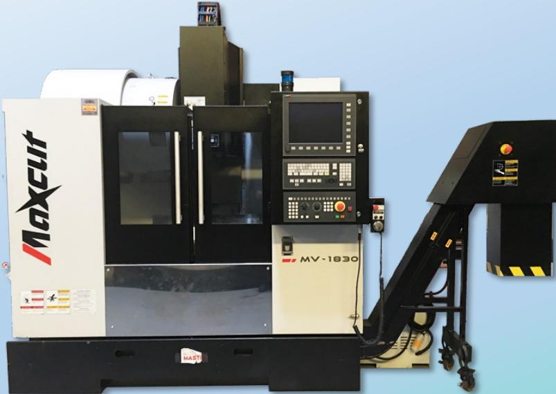
... including through spindle coolant / around spindle coolant / wash down coolant / coolant gun / steel belt lift-up chip conveyor / tool + part probe / Fagor 8065 POWER simultaneous 5-axis control / dynamic rotation tool centre point / kinematics machine calibration / FCAS real time monitoring and collision avoidance ...
